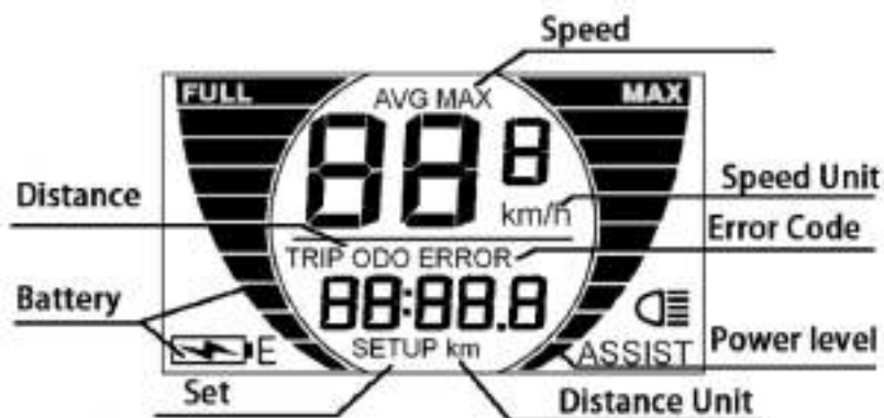
KM529 Monitor Area
