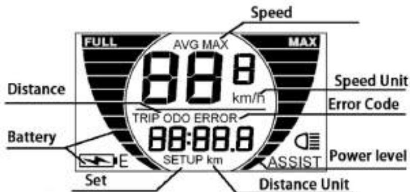
KM529 Monitor Area
